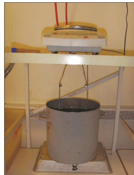
Figure 6. Installation of hydrostatic weighing
